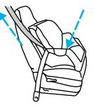
snugness of the child seat to the vehicle. Sometimes, a slight lean towards the buckle will additionally help to remove remaining slack from the belt.
